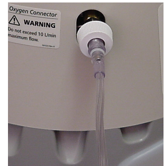
Figure 10: DISS Nut and Tailpiece connected to Reservoir Outlet
